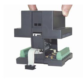
The jumpers are shown at right. Change the jumper settings as required, in accordance with the tables shown on the next page.
